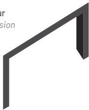
Cadre version angle recouvrement 60 mm Corner version frame covering 60 mm
