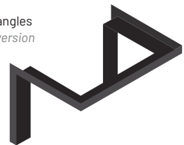
Cadre version angle recouvrement 15 mm Corner version frame covering 15 mm
